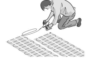
**6.** When embedding use cement-based tile adhesive, thinset mortar, screed or concrete, suitable for heated floors with good heat conductivity. As a minimum the BLUE THERMAL MAT must be covered entirely by the adhesive/screed/mortar /concrete, but a thicker layer might be required to ensure mechanical floor stability. Follow the guidelines given by the manufacturer and ensure that the BLUE THERMAL MAT is fully embedded.
